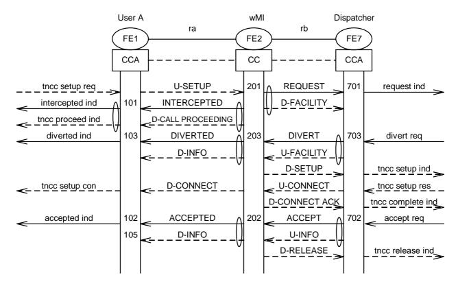
Figure 4: Successful interception with "on-demand" call set-up to the dispatcher
