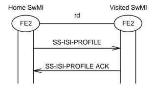
Figure 23: Supplementary service profile exchange
