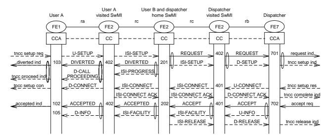
Figure 13: Authorization in home SwMI when user A and the dispatcher has migrated into different SwMIs
