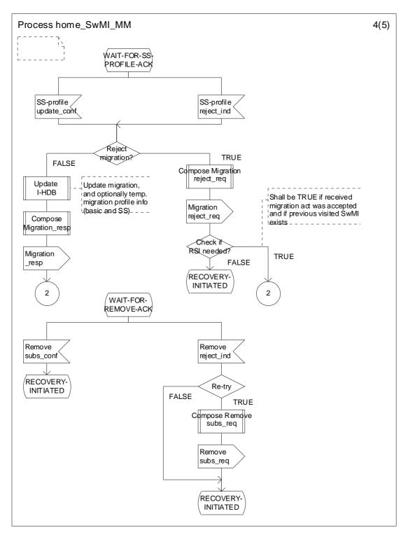
Figure B.1 (sheet 4 of 5): HMM recovery - dynamic description of the individual subscriber home SwMI MM
