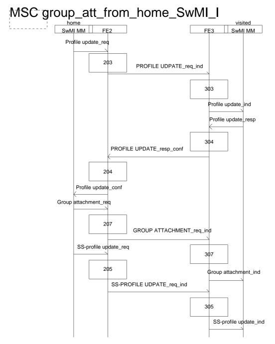
Figure 88: Rejection of group home SwMI MM initiated group attachment with migration profile exchange, rejected by subscriber
