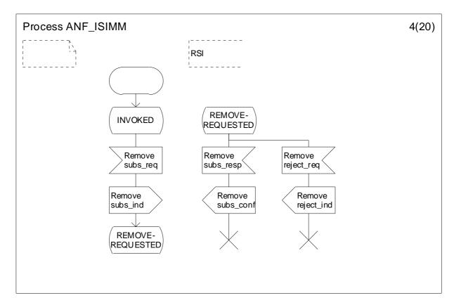
Figure 9: Dynamic description of RSI service using SDL
