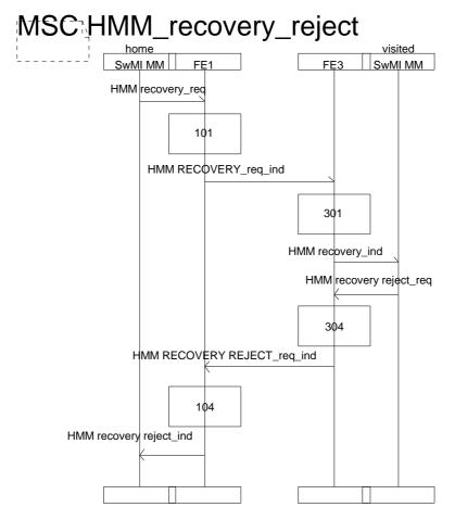
Figure 77: Rejection of HMM recovery
