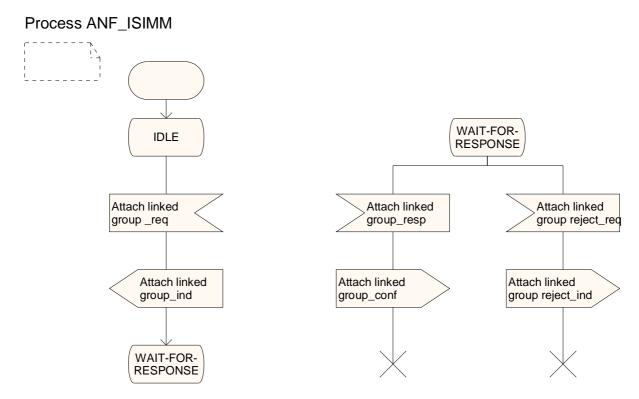
Figure 35b: Stage 1 SDL descriptions of the linked group attachment service when invoked from the group linking participating SwMI MM
