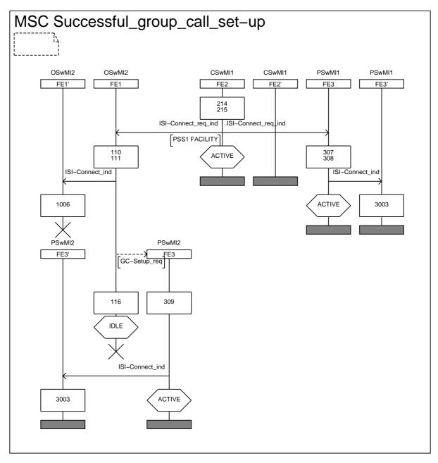
Figure 26: Information flow sequence - successful group call set-up, case 2 and 3 (sheet 4 of 4)
