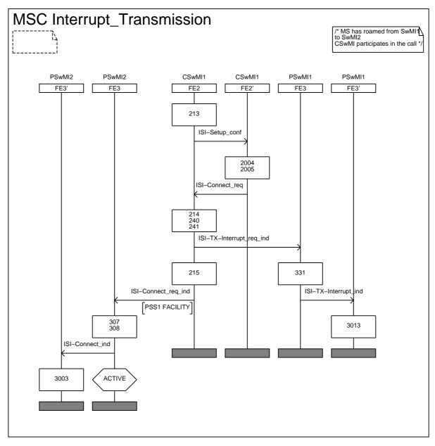
NOTE: If the parameter value, transmission grant in the ISI\_TX\_INTERRUPT PDU, is set to "transmission not granted", then an ISI\_RESOURCE PDU shall be sent to all participating SwMI(s) to check if resources are still available before an ISI\_TX\_GRANTED PDU is sent from the controlling SwMI. See figures 46 and 47 for an ISI\_RESOURCE PDU sequence.
