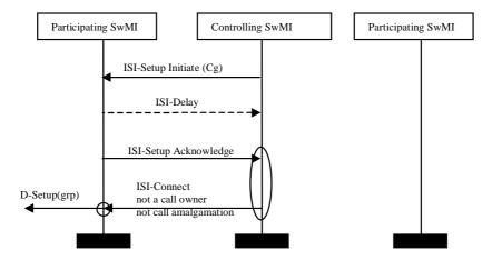
NOTE: A CSwMI may, at any time after call connection, send an ISI-SETUP INITIATE PDU to a SwMI which was not part of the original call but on which group members have since attached. This action may be triggered, for example, by the expiration of a timer causing the CSwMI to re-evaluate the list of PSwMIs, or by the attachment of an MS. It constitutes the ISI part of the Late Entry Supplementary Service. Each SwMI is responsible for operation of SS-LE within it.
