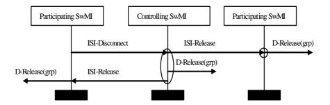
NOTE: The ISI-DISCONNECT PDU may be sent in either a PSS1-DISCONNECT or a PSS1-FACILITY message.
