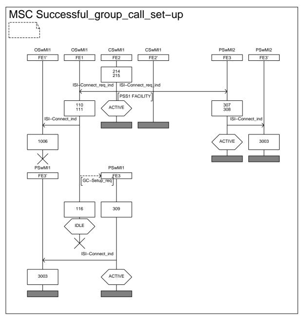
Figure 22: Information flow sequence - successful group call set-up, case 1 (sheet 3 of 3)
