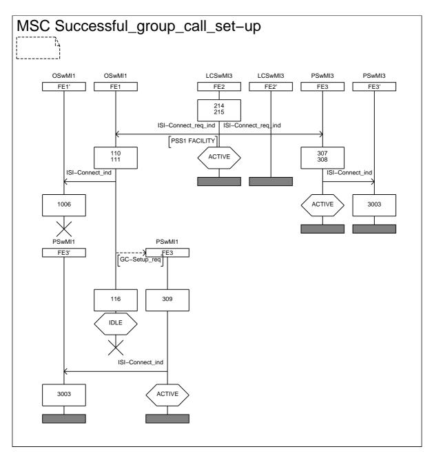
Figure 30: Information flow sequence - successful group call set-up, case 4 (sheet 4 of 4)
