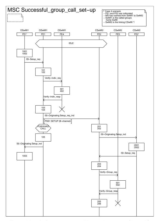
Figure 27: Information flow sequence - successful group call set-up, case 4 (sheet 1 of 4)
