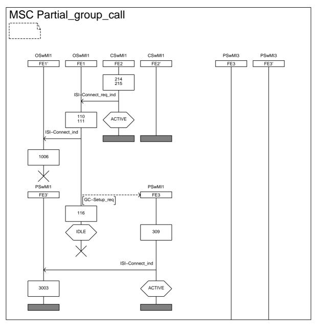
Figure 33: Information flow sequence - partial group call set-up (sheet 2 of 3)
