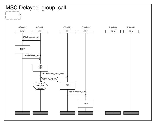
Figure 36: Information flow sequence - delayed group call set-up (sheet 2 of 4)
