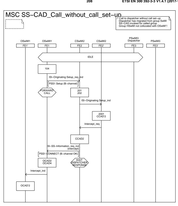
Figure B.6: Information flow sequence - Call to dispatcher without call set-up (sheet 1 of 3)
