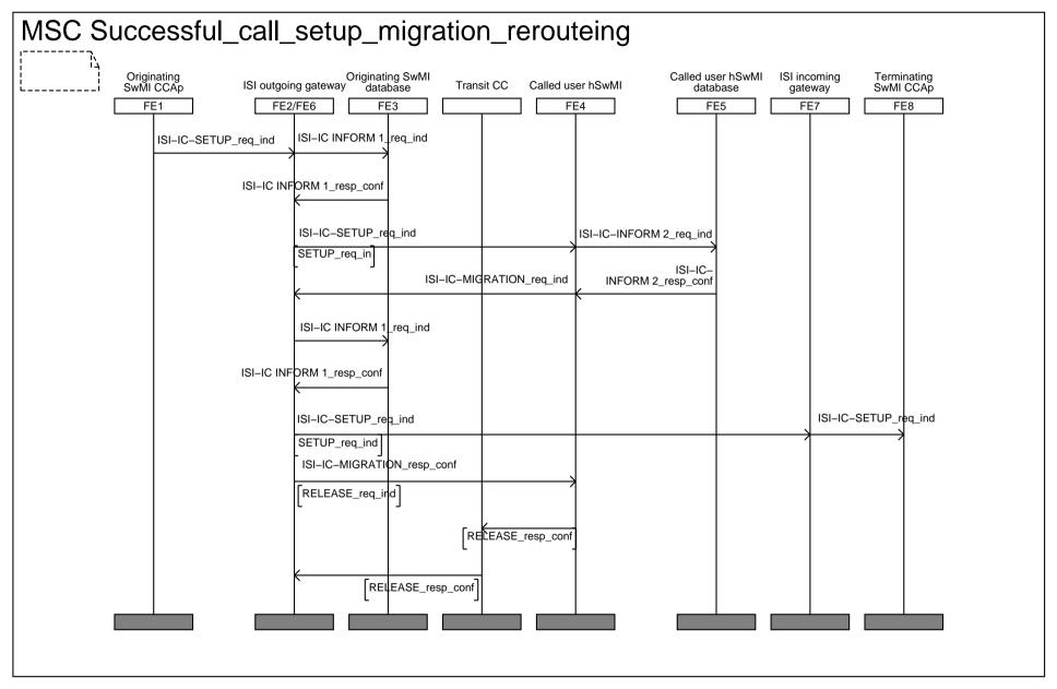
Figure 12: Information flow sequence - call set-up to a called user having migrated from SwMI B, using re-routeing
