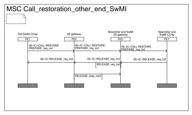
Figure 20: Information flow sequence - call restoration of an established inter-TETRA call in the other end SwMI
