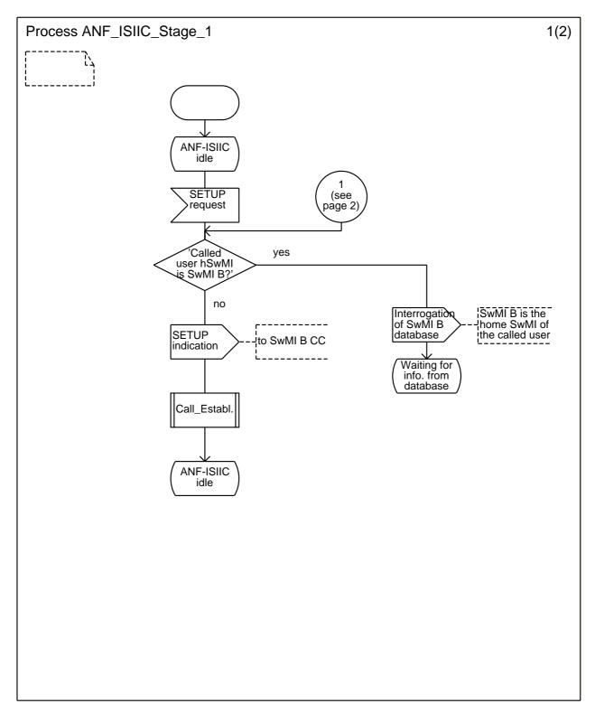
Figure 2 (sheet 1 of 5): ANF-ISIIC, overall SDL Main diagram
