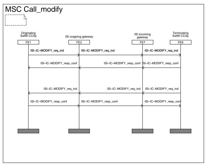
NOTE: The MODIFY information flows are not end-to-end between the originating and the terminating SwMI because they may result in a change in the 8 kbit/s encoding of the user information at the ISI, i.e. if the circuit mode service is modified, i.e. from speech to data service or vice-versa, or if the circuit mode service being data service, this service is changed, e.g. from 7,2 kbit/s to 4,8 kbit/s.
