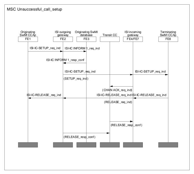
NOTE: The call set-up may also be rejected directly by the called SwMI, e.g. when it cannot match the air interface security level requested for the call. The corresponding information flow sequence has not been shown because it can easily be derived from figure 15.
