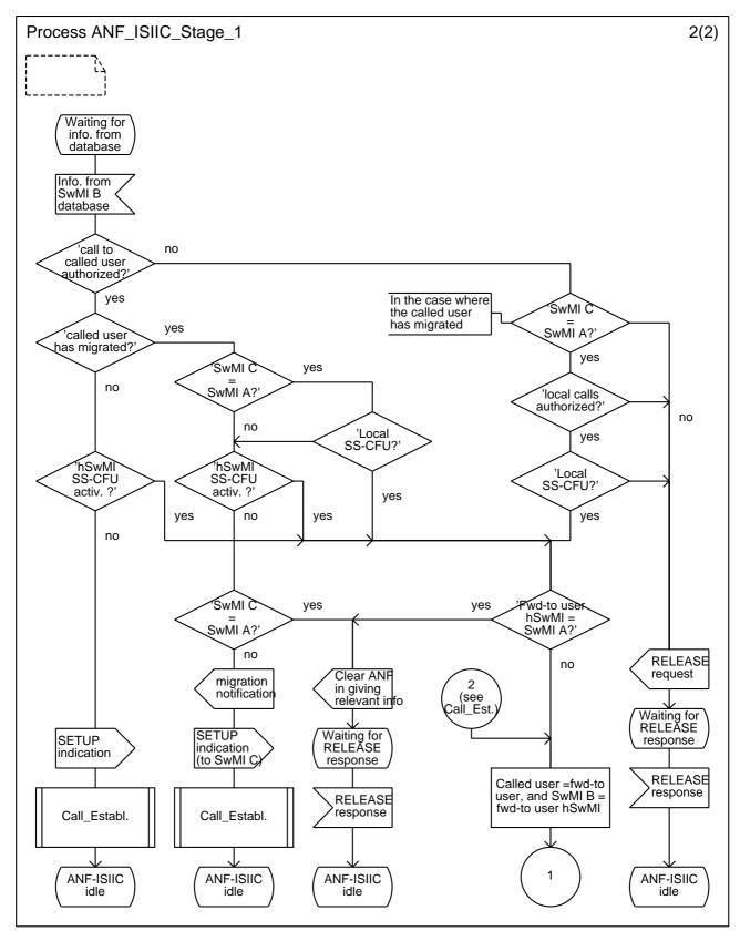
Figure 2 (sheet 2 of 5): ANF-ISIIC, overall SDL Main diagram
