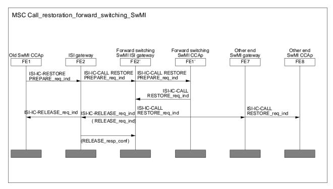
Figure 19: Information flow sequence - call restoration of an established inter-TETRA call in the forward switching SwMI
