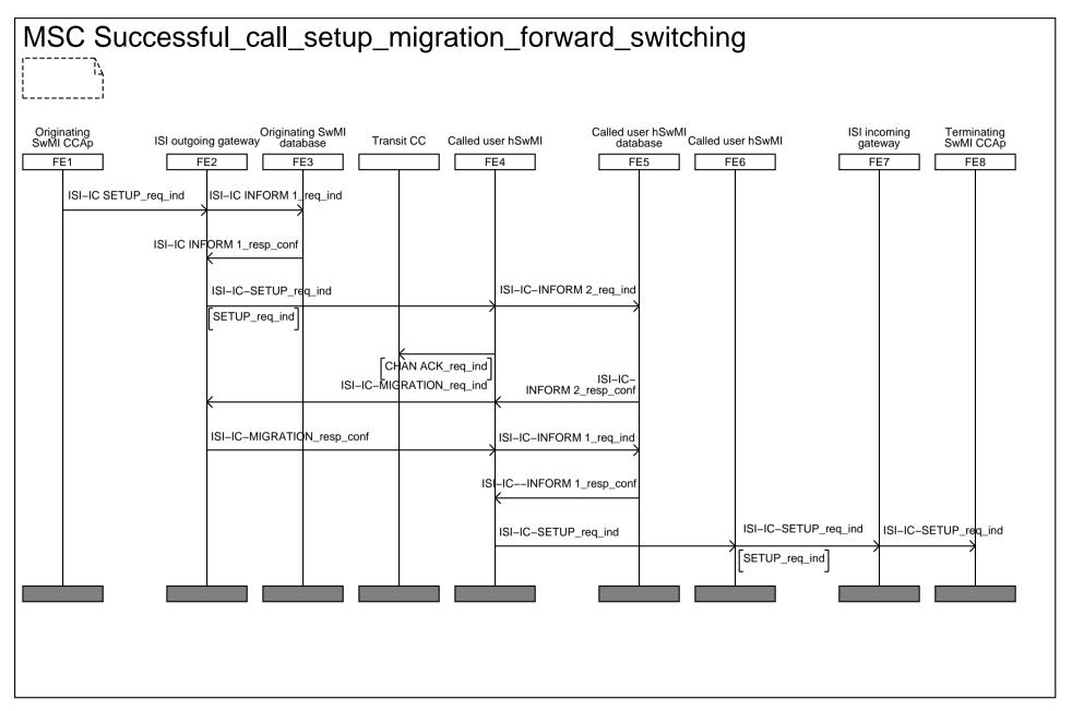
Figure 11: Information flow sequence - call set-up to a called user having migrated from SwMI B, using forward switching
