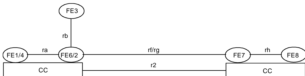
Figure 5: Example relationship between models for ANF-ISIIC and basic call in the case of called user hSwMI being SwMI B, with no migration
