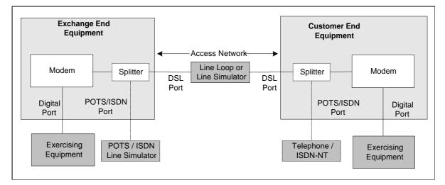
Figure 3: DSL Access System Configuration
