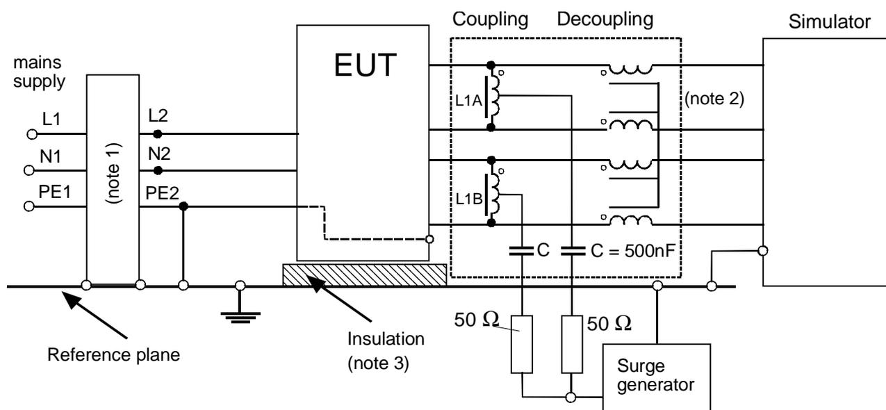
NOTE 1: The impedance matching network is used to decouple the mains and to provide low impedance to reference plane at EUT side. The impedance matching network is described in figure A.2.
