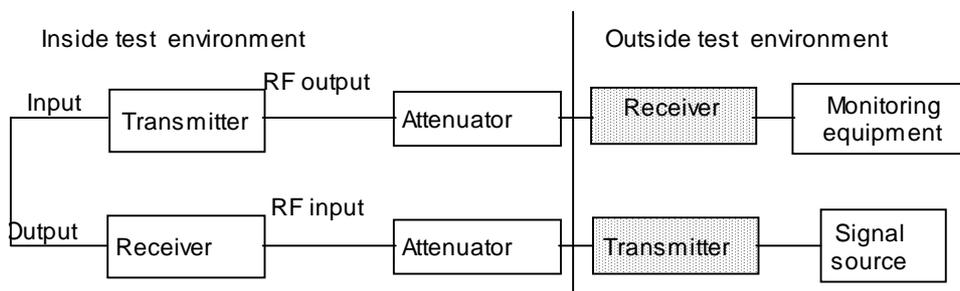
**Figure 6: Test configuration of transceivers**
