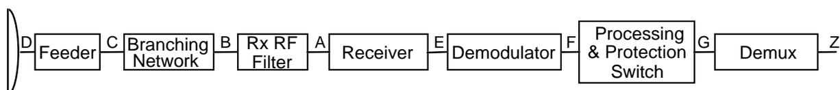
NOTE 1: For the purposes of defining the reference points, the branching network (B to C) does not include a hybrid.
