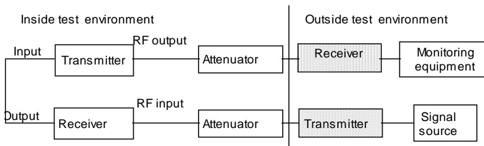
**Figure 6: Test configuration of transceivers**
