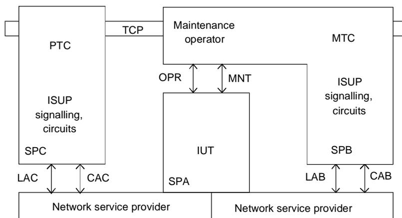
**Figure 4: ISUP test configuration for intermediate exchanges**
