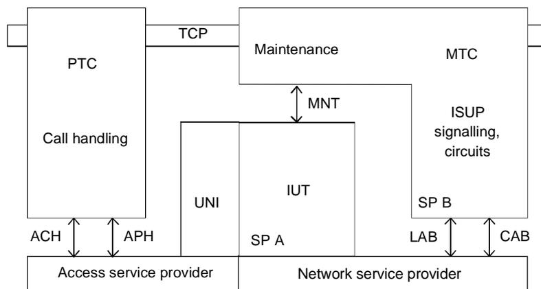
**Figure 6: ISUP test configuration for local exchanges**
