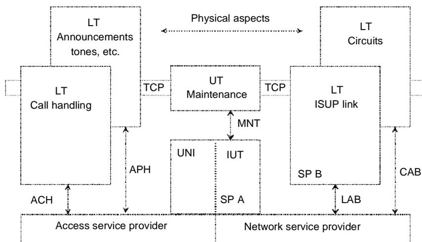
**Figure 5: ISUP test method for originating/destination exchanges**
