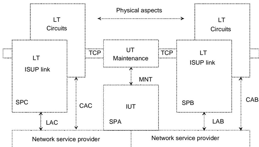
**Figure 3: ISUP test method for intermediate exchanges**
