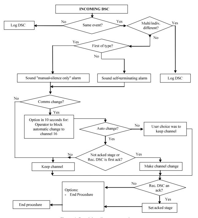
Figure 4: Receiving distress procedure
