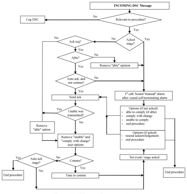
Figure 8: Receiving non-distress procedure
