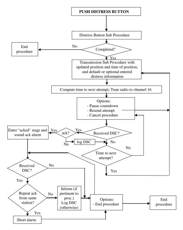
Figure 1: Sending distress procedure
