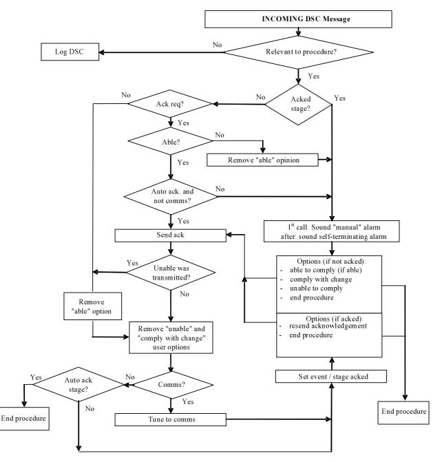
Figure 8: Receiving non distress procedure
