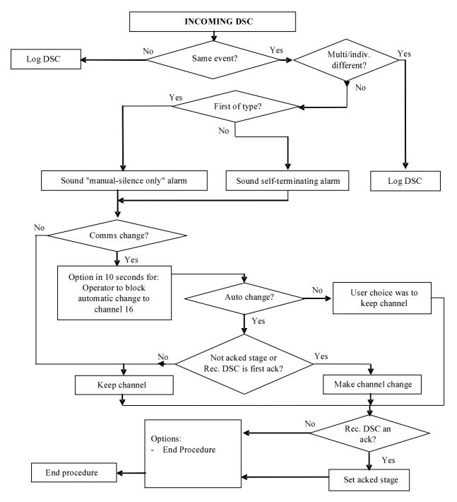
Figure 4: Receiving distress procedure
