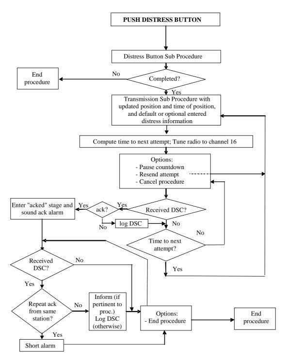
Figure 1: Sending distress procedure
