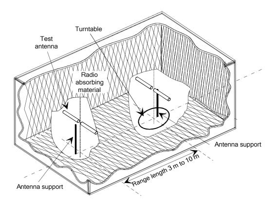
Figure A.1: A typical anechoic chamber
