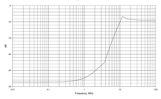
Figure F.1: Conversion factor C<sub>30</sub> versus frequency
