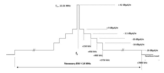
Figure G.3: Spectrum mask limit for wideband RFIDs in the 13,56 MHz range
