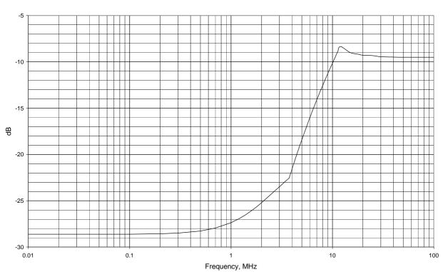
Conversion factor,  $C_{30}$ , for limits at 30 m distance, dB
