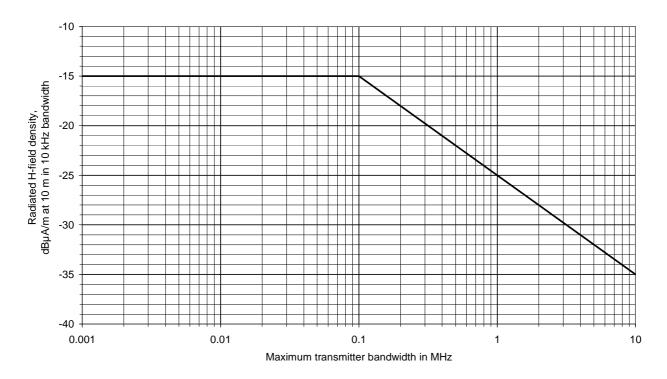
Figure K.1: Radiated bandwidth and H-field density at 10 m distance
