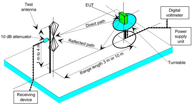
Figure D.4: Measuring arrangement on ground plane test site (OATS set-up for spurious emission testing)
