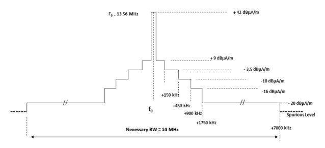
Figure J.3: Spectrum mask limit for wideband RFIDs in the 13,56 MHz range
