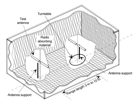
Figure D.1: A typical anechoic chamber
