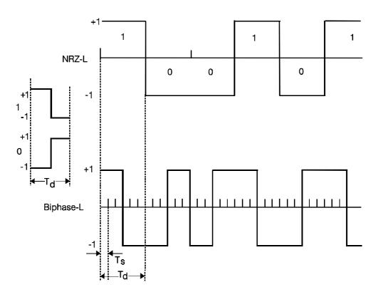
Figure 2: Example of bi-phase-L coding
