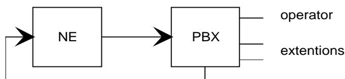
Originating accesses to NE are at PCM span level, with e.g. touch tone register signalling and R2 digital line signalling.(\*).
