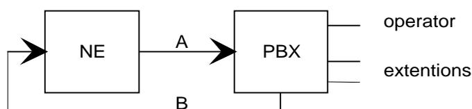
Accesses A are PCM spans using e.g. MFC register signalling and R2 digital line signalling (\*).
