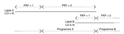
Figure 11: PRF to signal precise start times
