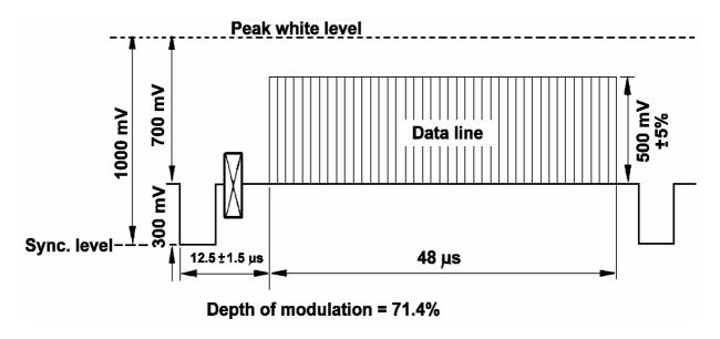
Figure 8: Insertion of the data line into the video signal
