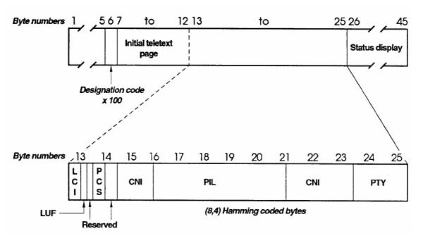
Figure 7: Structure of the Teletext data packet 8/30 format 2
