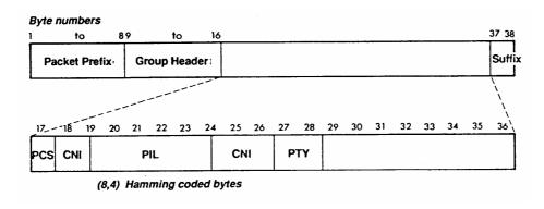
Figure C.1: Structure of the programme delivery data in DIDON III
