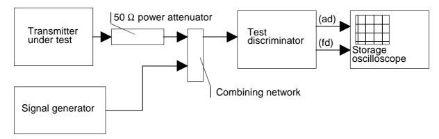
Figure 2: Measurement arrangement
