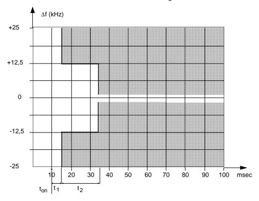
Switch off condition: limits:  $\Delta f \leq$  25 kHz during  $t_3^{}$  (= 5 msec)
