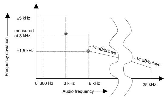
Figure 1: Frequency deviation versus audio modulation frequency
