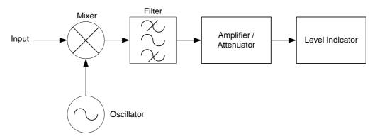
Figure A.1: Power measuring receiver
