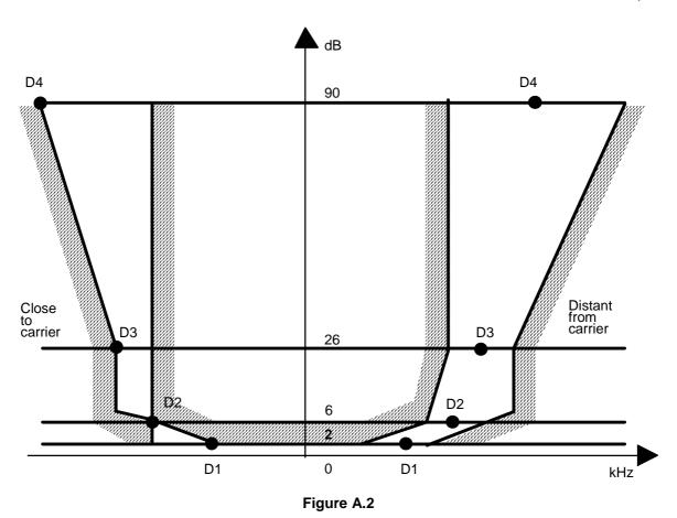
The selectivity characteristics shall keep the following frequency separations from the nominal centre frequency of the adjacent channel given in table A.1.
