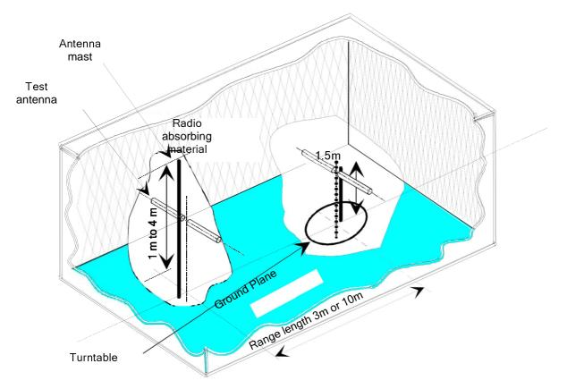
Figure B.2: A typical anechoic chamber with a conductive ground plane
