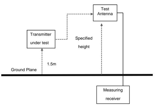
Figure 1: Measurement arrangement
