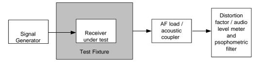
Figure B.6: Measuring arrangement for calibration
