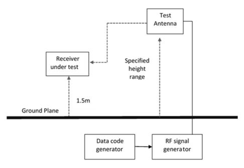
Figure 10: Measuring arrangement
