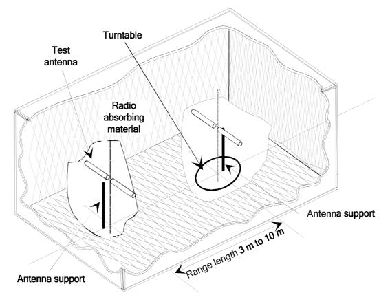
Figure B.1: A typical anechoic chamber
