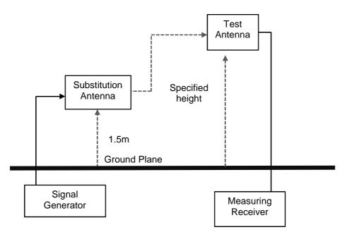
Figure 2: Substitution measurement arrangement
