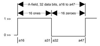
Figure 27: Test packet structure for case 2, A-field
