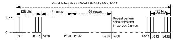
NOTE: Bits  $b_0$  to  $b_{127}$  and  $b_{512}$  to  $b_{639}$  are alternating 1s and 0s.
