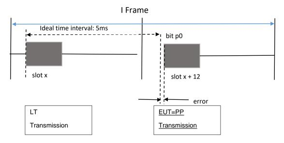
Figure 24: PP packet transmission error definition
