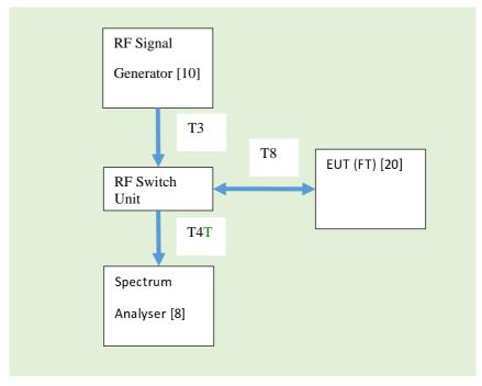
Figure 32: FT Test Setup
