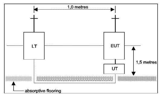
Figure 16: Test arrangement
