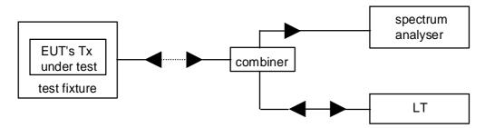
Figure 6: Measuring arrangement for calibration
