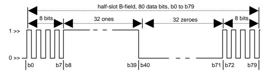
NOTE: Bits  $b_0$  to  $b_7$  and  $b_{72}$  to  $b_{79}$  are alternating 1s and 0s with the even order bits ( $b_0$ ,  $b_2$ ,  $b_4$ , etc.) set to "1" and the odd-order bits ( $b_1$ ,  $b_3$ ,  $b_5$ , etc.) set to "0".
