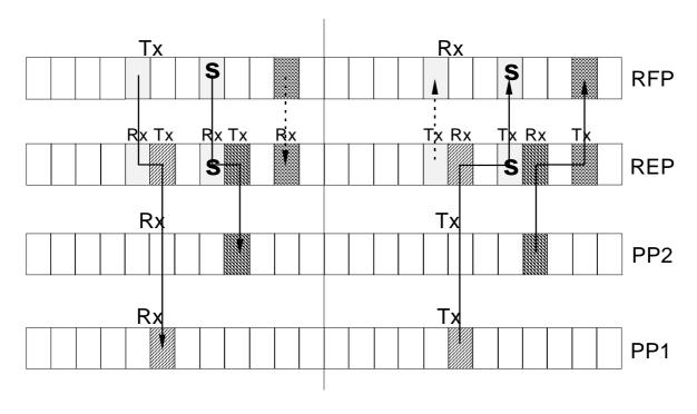
Figure 40: Two single duplex bearer connections, REP relayed with interlacing
