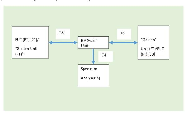
Figure 34: Channel Release Test Setup
