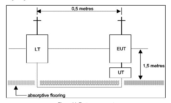
Figure 14: Test arrangement
