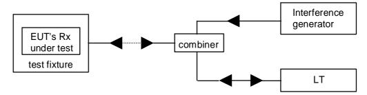
Figure 7: Measuring arrangement for calibration
