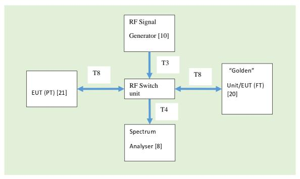
Figure 33: PT Test Setup
