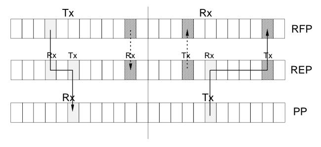
Figure 38: Frame multiplexing structure when relaying one duplex bearer connection through a single hop
