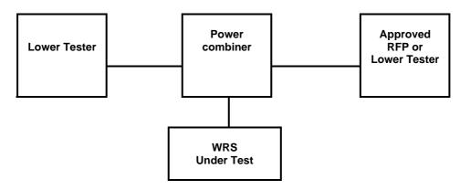
Figure 36: WRS testing as an RFP
