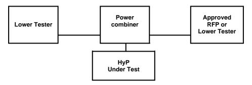
Figure 44: HyP testing as an RFP
