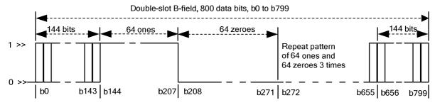
NOTE: Bits  $b_0$  to  $b_{143}$  and  $b_{656}$  to  $b_{799}$  are alternating 1s and 0s.
