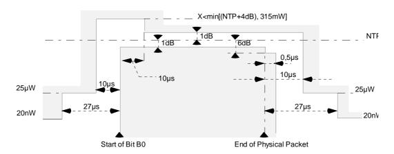
Figure 25: Physical packet power-time template
