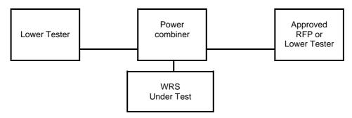
Figure 42: WRS testing as an RFP
