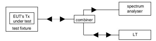
Figure 6: Measuring arrangement for calibration
