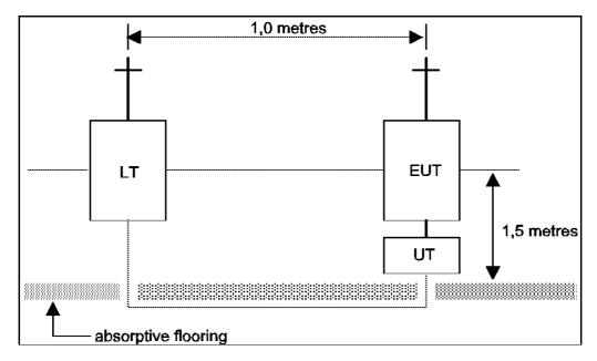
Figure 17: Test arrangement
