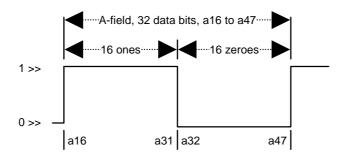
Figure 30: Test packet structure for case 2, A-field
