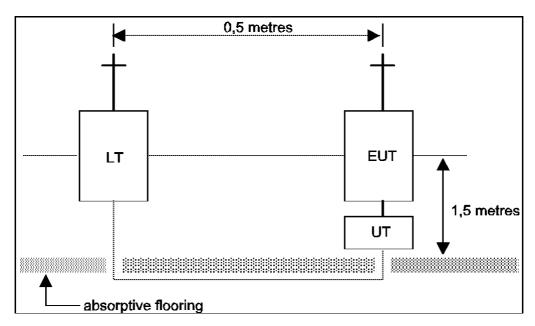
Figure 15: Test arrangement
