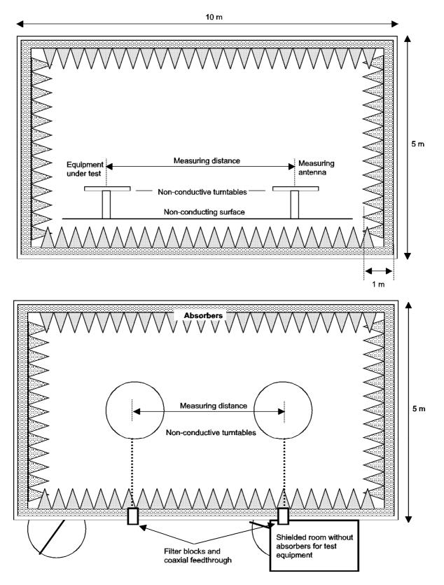
Figure 5: Example of construction of an anechoic chamber
