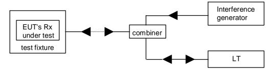
Figure 7: Measuring arrangement for calibration
