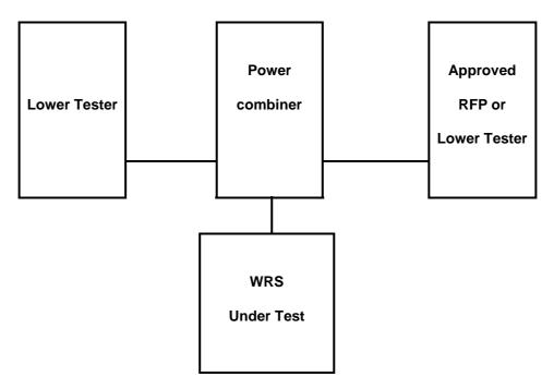
Figure 35: WRS testing as an RFP
