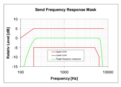
Figure 7.11: Send frequency response mask
