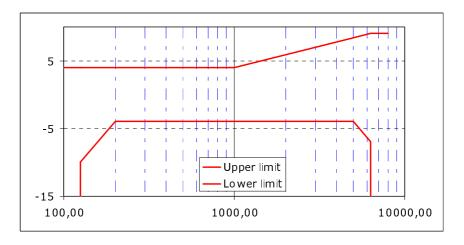
Figure 7.15: Sending sensitivity/frequency mask for HFT
