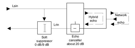
Figure A.4: Implementation of the network echo control 2-wire line interface
