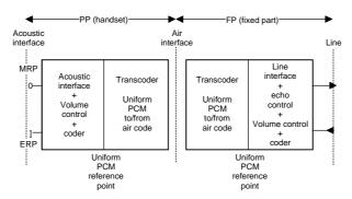
Figure 4.1: Basic reference configuration
