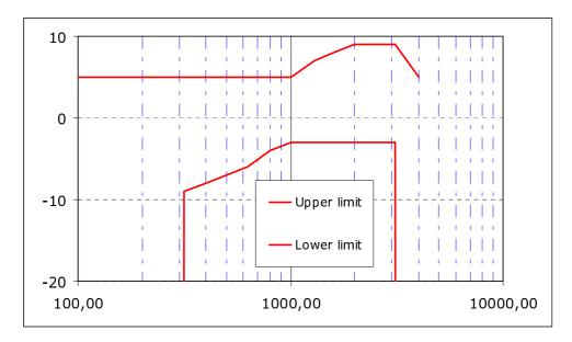
Figure 7.7: Sending sensitivity/frequency mask for HFT
