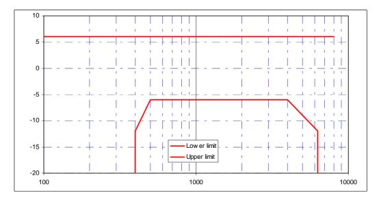
Figure 7.18: Receiving sensitivity/frequency mask for standard hand-held PP
