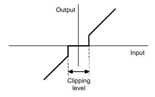
Figure A.2: Transfer function of non-linear processor
