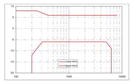
Figure 7.16: Receiving sensitivity/frequency mask for Desktop handsfree PP
