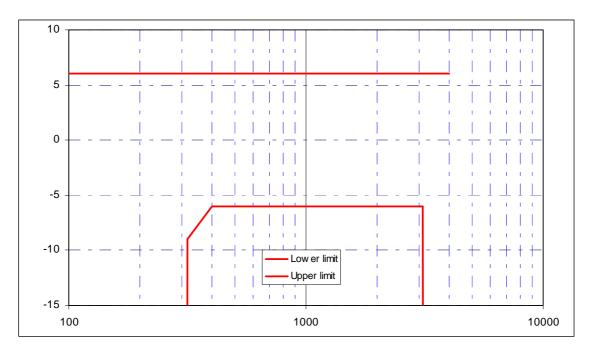
Figure 7.8: Receiving sensitivity/frequency mask for Desktop hands-free PP
