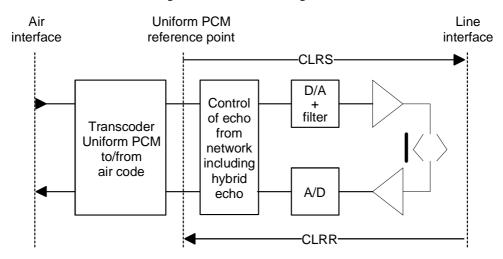
Figure 4.5: FP with an analog interface
