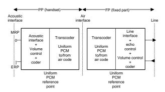
Figure 4.1: Basic reference configuration
