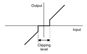
Figure A.2: Transfer function of non-linear processor
