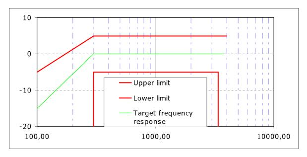
Figure 7.3: Send frequency response mask for PP types 1c and 1d
