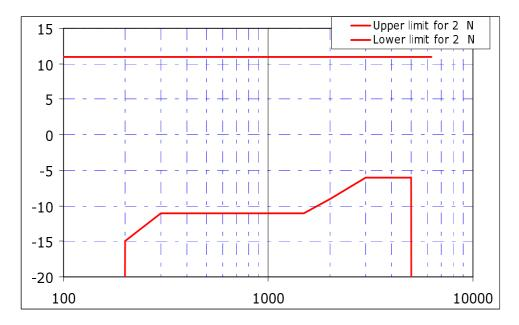
Figure 7.14: Receive frequency response mask for 2 N application force
