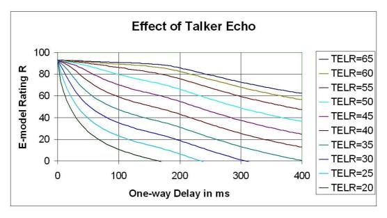
Figure E.1: E-model rating versus delay and TELR
