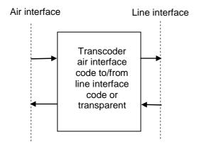
Figure 4.4: FP simplified functional model without optional functions
