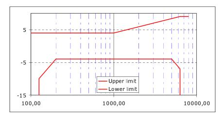
Figure 7.15: Sending sensitivity/frequency mask for HFT
