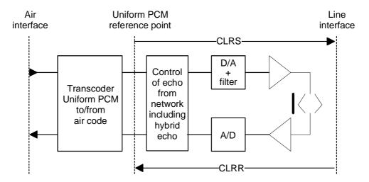
Figure 4.5: FP with an analog interface
