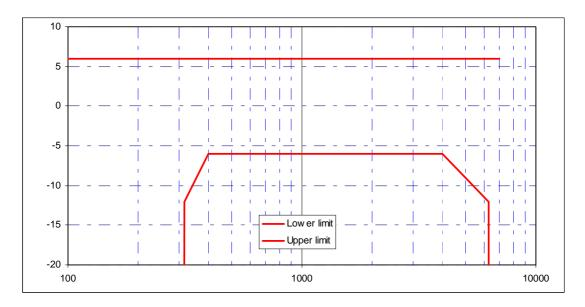
Figure 7.17: Receiving sensitivity/frequency mask for improved handheld PP
