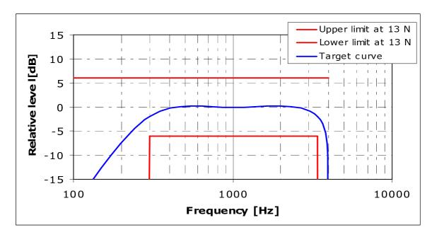
Figure 7.5: Receive frequency response mask for 13N application force
