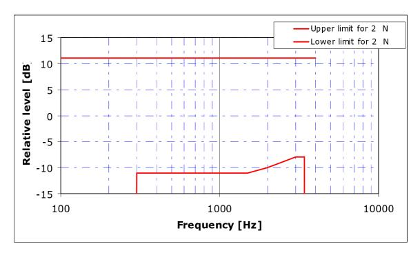
Figure 7.6: Receive frequency response mask for 2 N application force
