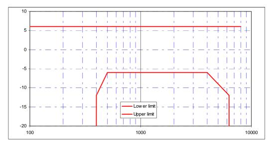
Figure 7.18: Receiving sensitivity/frequency mask for standard hand-held PP
