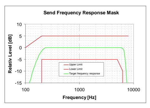
Figure 7.11: Send frequency response mask
