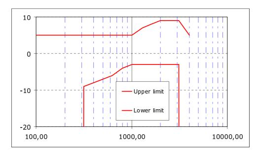
Figure 7.7: Sending sensitivity/frequency mask for HFT
