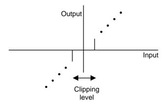
Figure A.2: Transfer function of non-linear processor
