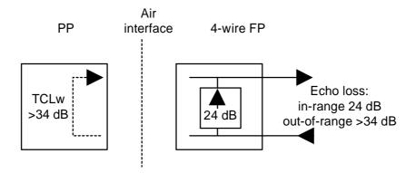
NOTE: The artificial echo simulates the echo from a very good analog 2-wire telephone. When a public network operator uses an echo canceller in the network (e.g. for a satellite link), the artificial echo loss path provides an in-range echo to ensure that the echo canceller and its Non-Linear Processor (NLP) is active. The NLP cancels the 34 dB DECT handset echo. See annex A, clause A.1.1.
