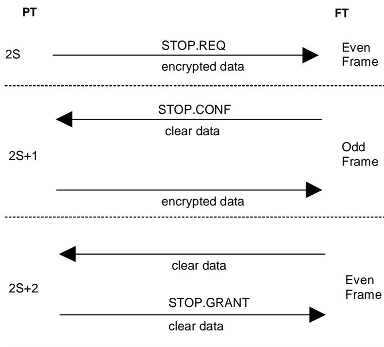
**Figure 6.8: Encryption stop - good link example**
