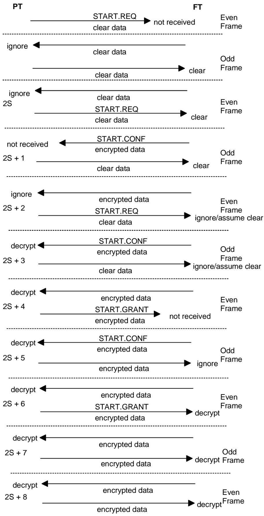
Figure 6.7: Encryption start - poor link example
