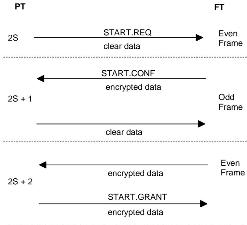
**Figure 6.6: Encryption start - good link example**
