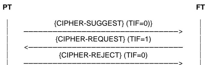
**Figure H.8: PT initiated cipher switching, case 3**
