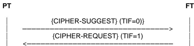
**Figure H.6: PT initiated cipher switching, case 1**
