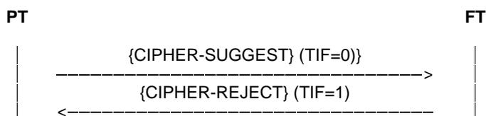
**Figure H.7: PT initiated cipher switching, case 2**
