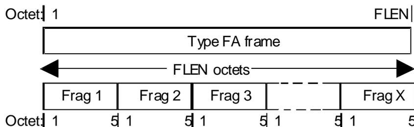
**Figure 6.1.4.2.1: C<sub>S</sub>/CL<sub>S</sub> logical channel fragmentation**
