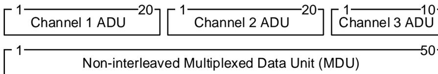
**Figure 11.6.2.3.1: Example of non-interleaved packing (MCS Ref: P2/16)**
