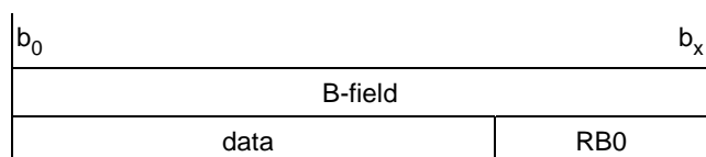
Figure 6.13: B-field structure of the Singlesubfield protected format
