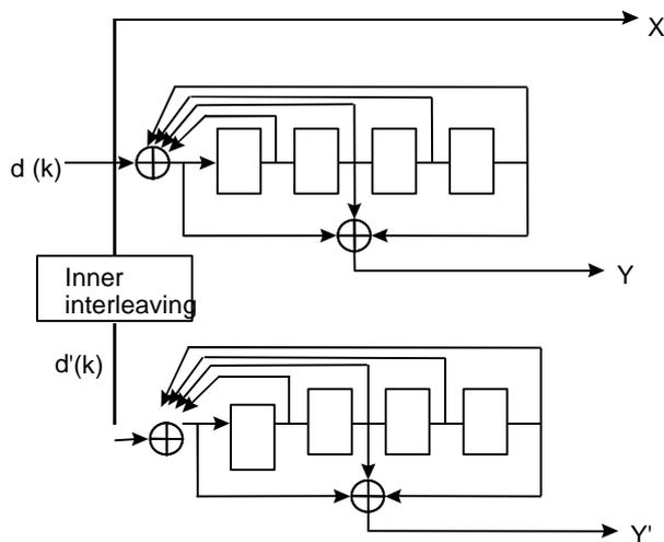
**Figure I.4: FOCTC structure**
