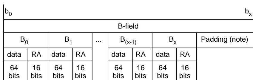
**Figure 6.12: B-field structure of the Multisubfield protected format**
