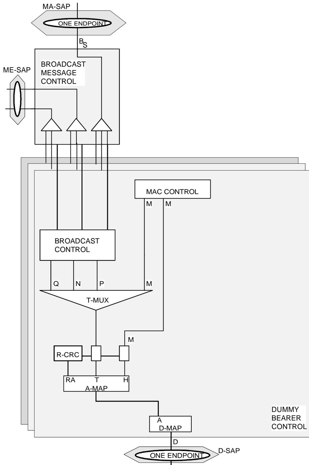
Figure 6.3: DBC multiplexing
