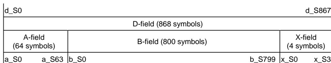
Figure 6.6: A-field, B-field and X-field in the D-field
