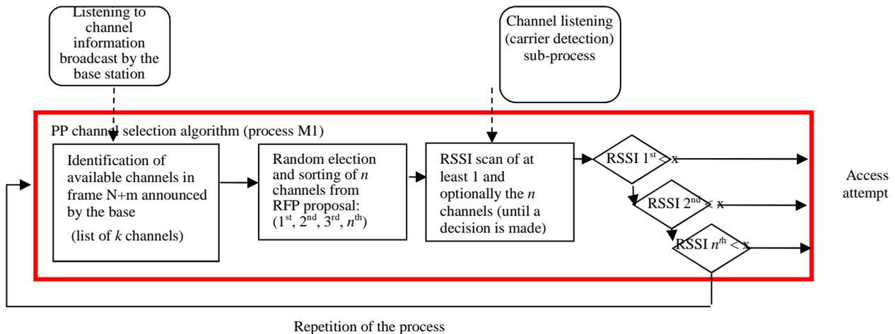
**Figure 11.3: Internal diagram of Channel Selection Process M1 (PP side channel selection process)**
