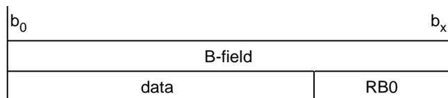
**Figure 6.13: B-field structure of the Singlesubfield protected format**
