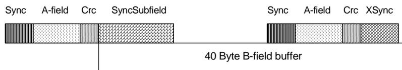
**Figure 9.5: Example: full slot contains normal dummy**
