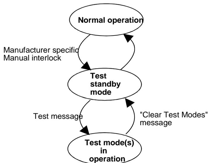
Figure 12.1: State mode diagram for IUTs during testing
