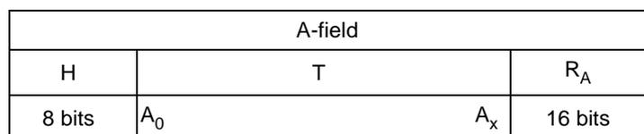
Figure 6.10: A-field mapping
