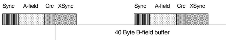
**Figure 9.4: Example: full slot contains 2 or 3 DummyPointer**
