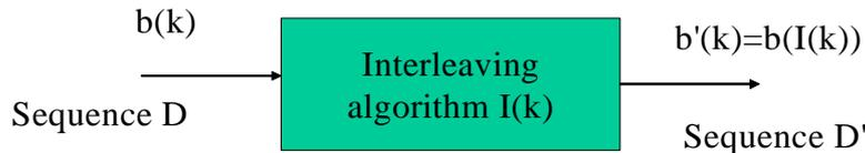
**Figure I.5: Inner interleaving rule principle**
