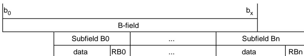
**Figure 6.13d: B-field structure of the constant-size subfield protected format for any other higher level modulation**
