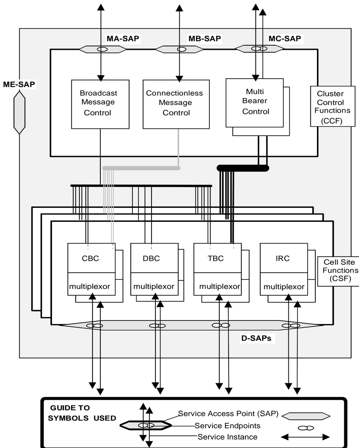
NOTE: MA, MB, MC and D are Service Access Points (SAPs) between the adjacent layers. Each line through these SAPs represents an independent service instance. ME is a SAP to the management entity.
