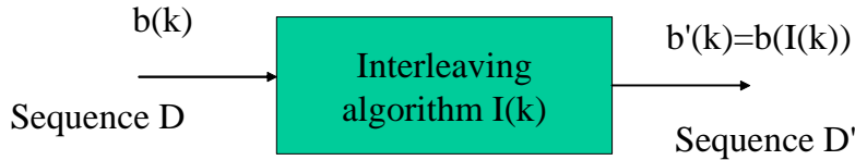
Figure I.5: Inner interleaving rule principle
