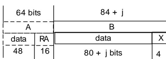
**Figure 6.22: Unprotected D08 B-field format (half slot, 2 level modulation)**
