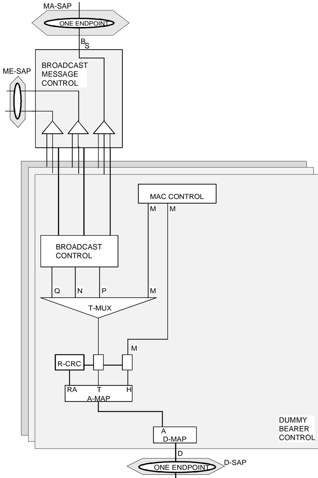
Figure 6.3: DBC multiplexing
