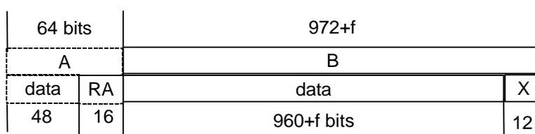
**Figure 6.21: Unprotected D96-field format (full slot, 8 level modulation)**
