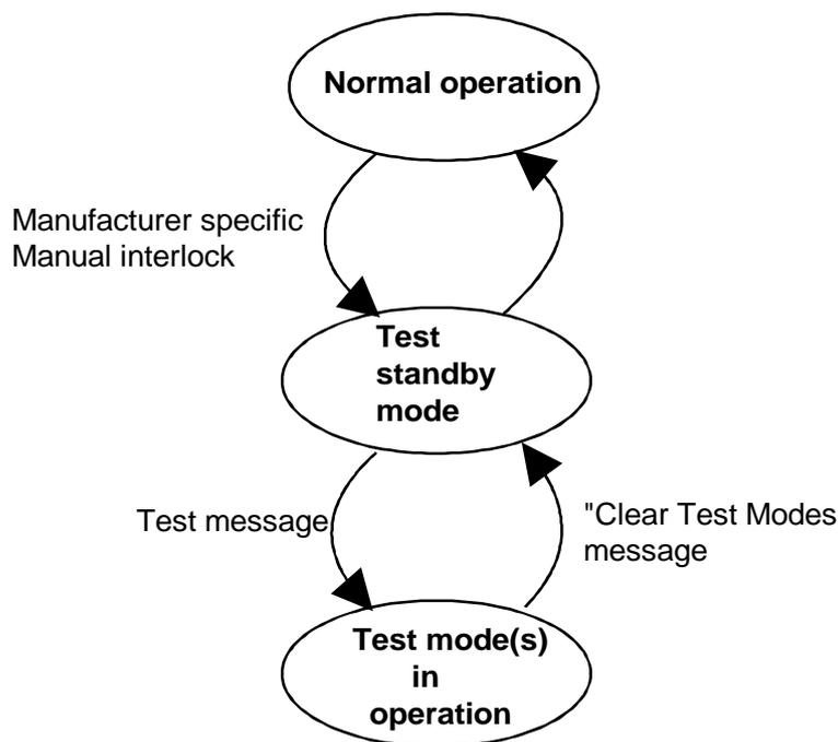
Figure 12.1: State mode diagram for IUTs during testing
