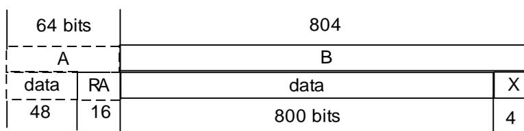
Figure 6.16: Unprotected D80 B-field format (double slot, 2 level modulation)
