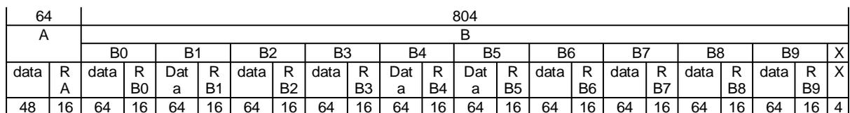
Figure 6.25: Multisubfield protected B-field format D80 (double slot, 2 level modulation)
