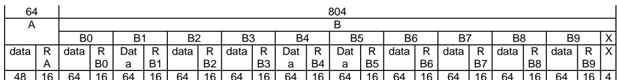
**Figure 6.25: Multisubfield protected B-field format D80 (double slot, 2 level modulation)**
