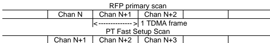
**Figure 11.1: PT receiver scan sequence**
