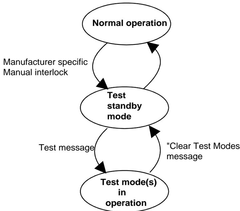
Figure 12.1: State mode diagram for IUTs during testing
