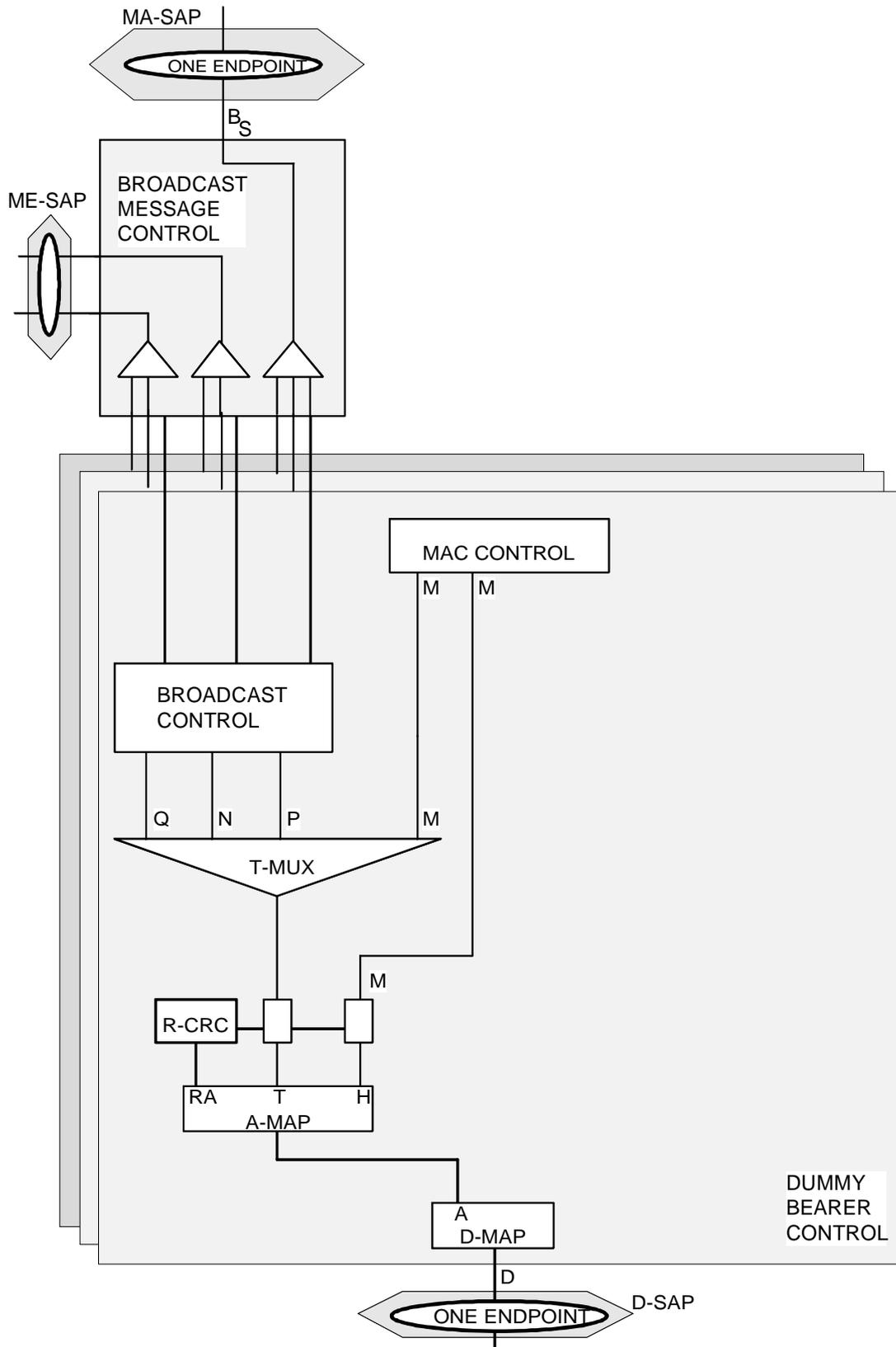
Figure 6.3: DBC multiplexing
