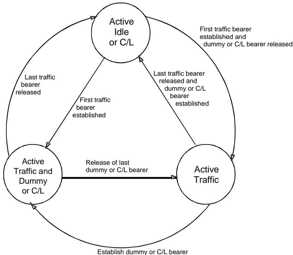
**Figure 4.8: RFP state diagram**
