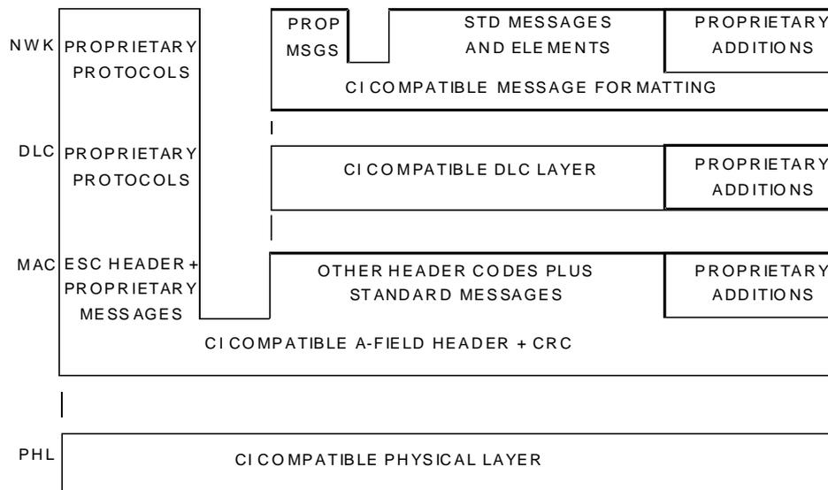
**Figure 2: Structure of escape routes within the CI**
