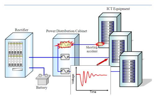
Figure G.1: Definition of transient voltage impact
