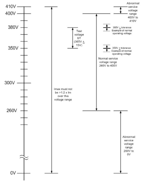
Figure H.1: Diagram of voltage ranges and values at the interface A3
