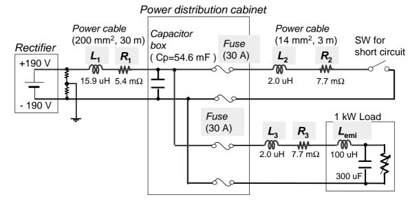
Figure G.2: Example of simulation circuit for short circuit and voltage transient measurement
