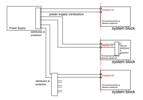
NOTE: The figure is a drawing of the power system and does not show the PE conductor.
