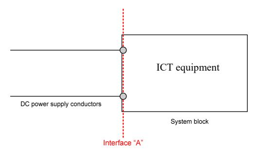
Figure 1: Identification of interface "A"
