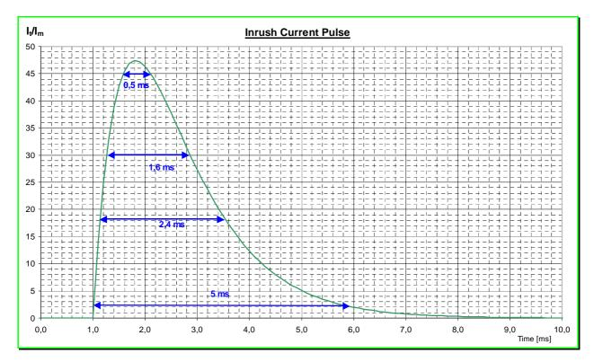
Figure C.1: Example of current pulse and associated measurements
