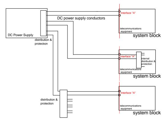
Figure A.1: Identification of interface "A" (examples)
