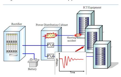
Figure G.1: Example of transient voltage impact
