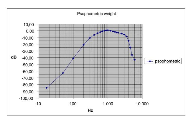
Figure E.1: Psophometric filter frequency response
