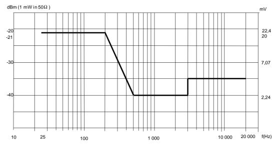
Figure 6: Maximum levels of narrowband noise
