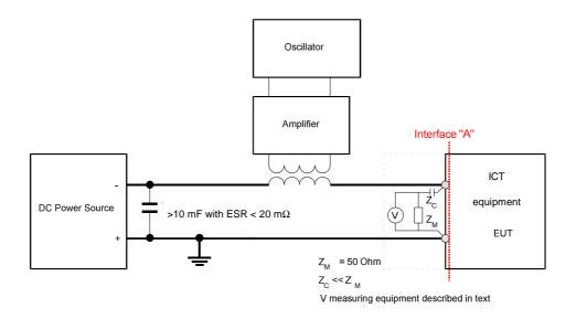
Figure 5: Example of a typical test arrangement for immunity measurement at interface "A"
