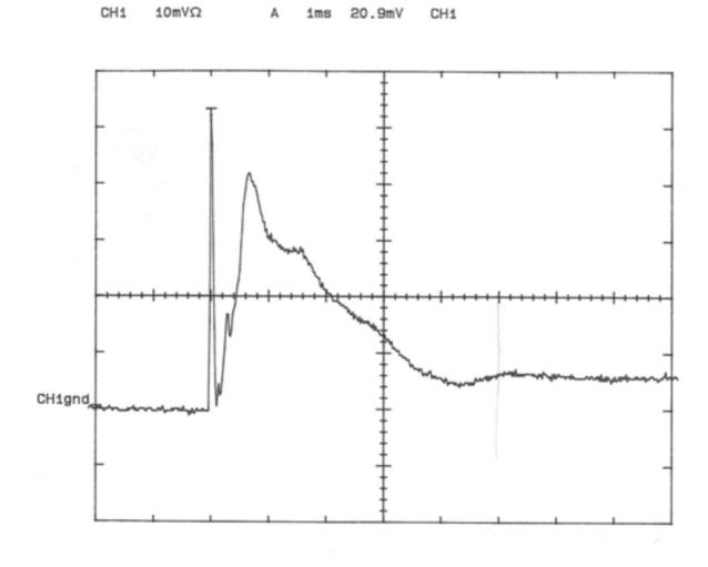
NOTE: In this example the inrush current measurement starting point is set at the beginning of the filter capacitor charging pulse.
