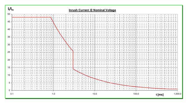
Figure 2: Maximum inrush current characteristics for ICT equipment at nominal voltage and maximum load
