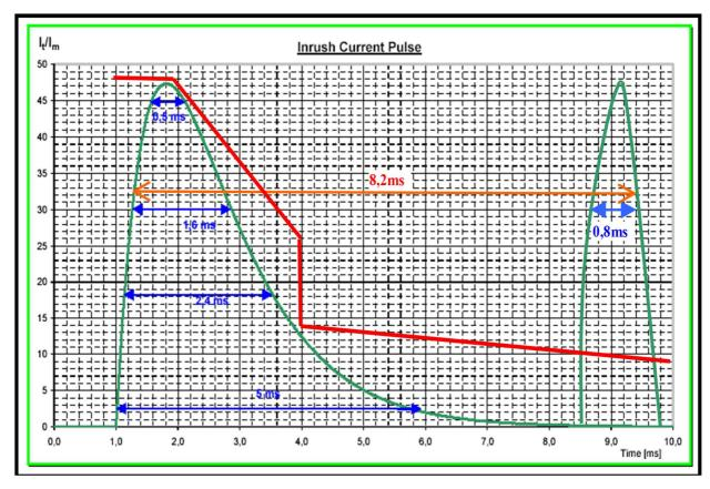
Figure C.3: The width obtained is the addition of the width of the individual pulses (1,6 ms + 0,8 ms)
