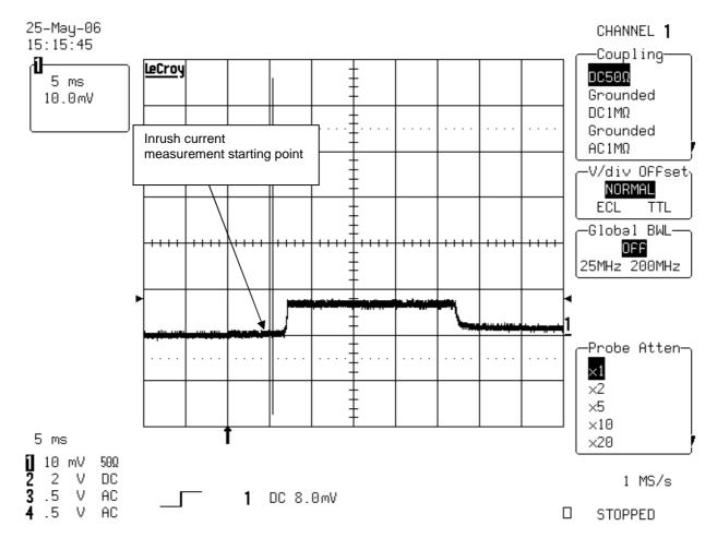
NOTE: In this example the inrush current measurement starting point is set at the beginning of the single pulse.
