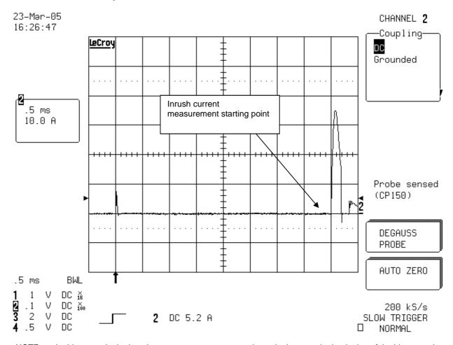
NOTE: In this example the inrush current measurement starting point is set at the beginning of the biggest pulse.
