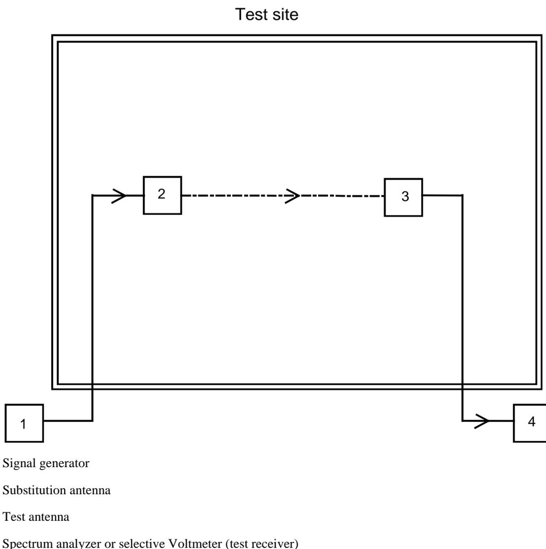
**Figure 10: Measurement arrangement**
