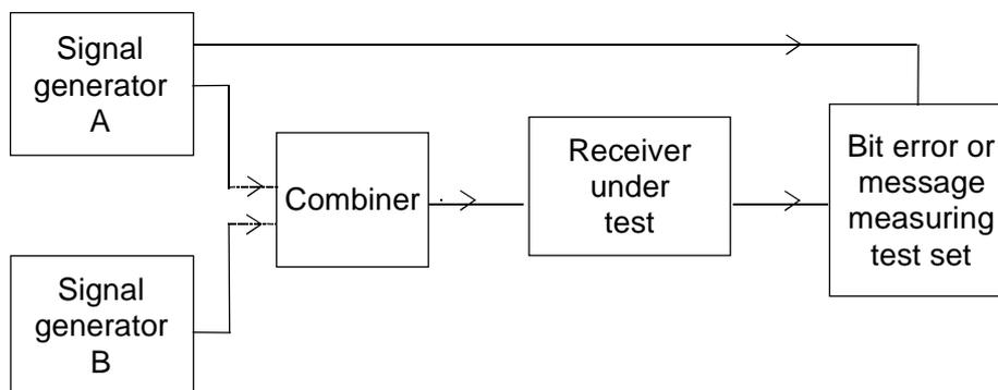
Figure 25: Measurement arrangement
