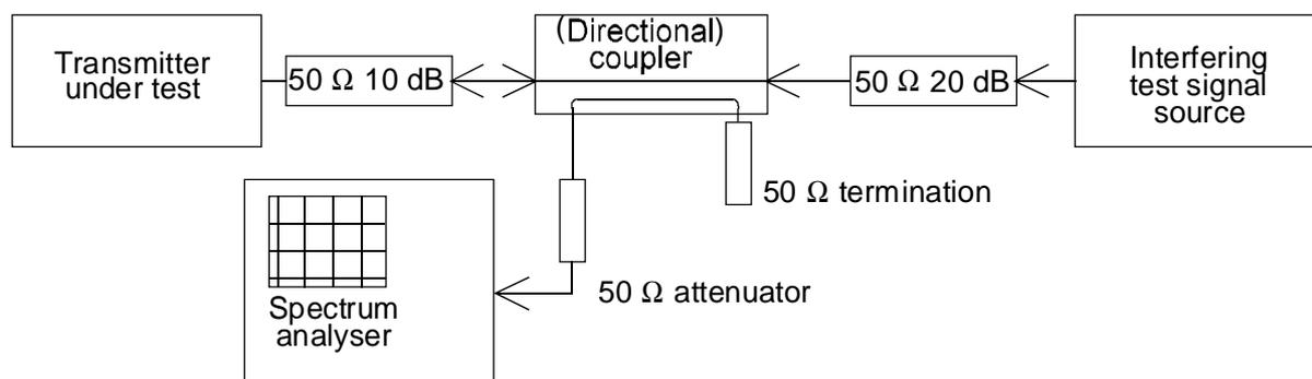
**Figure 11: Measurement arrangement**
