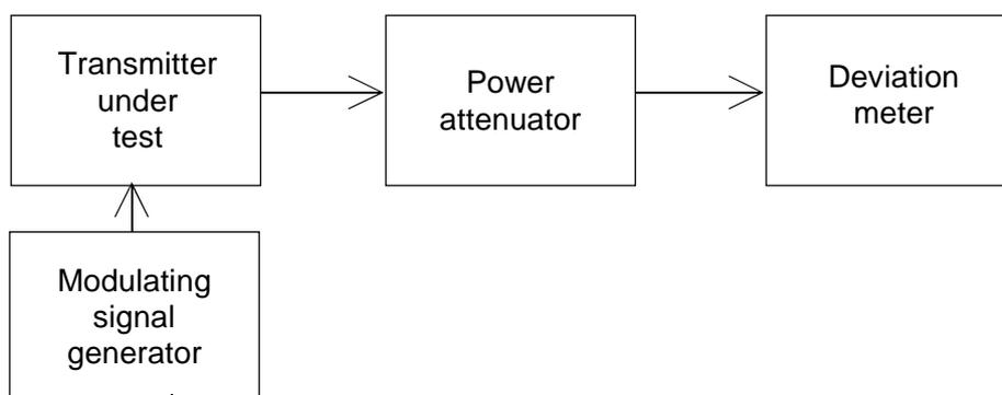
**Figure 6: Measurement arrangement**
