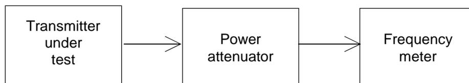
**Figure 2: Measurement arrangement**
