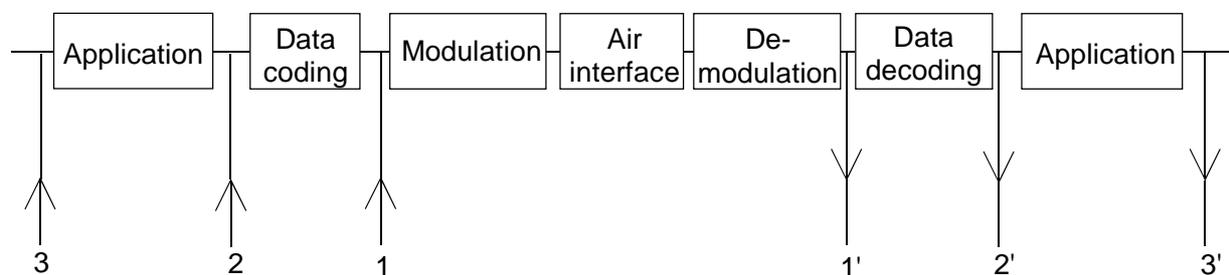
**Figure 1: Test points for bit stream measurements**
