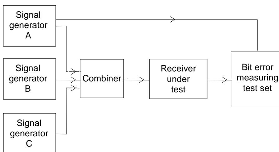
**Figure 26: Measurement arrangement**
