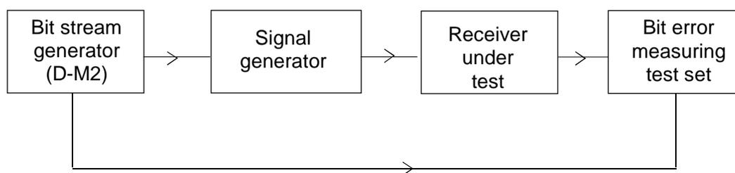
**Figure 19: Measurement arrangement**
