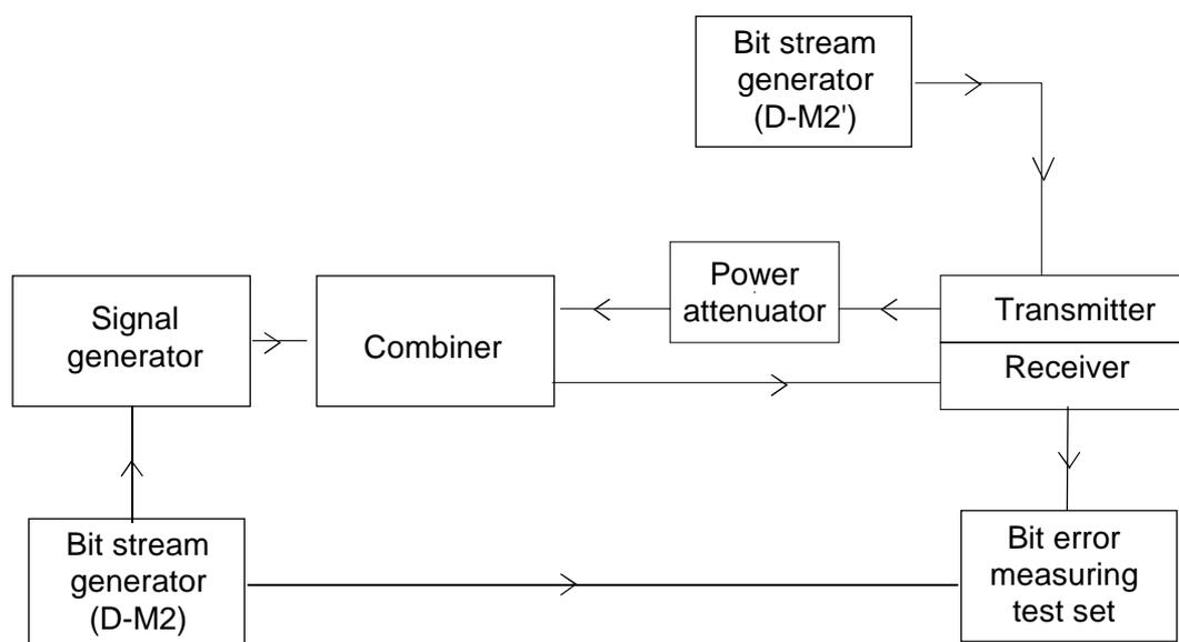
**Figure 34: Measurement arrangement**
