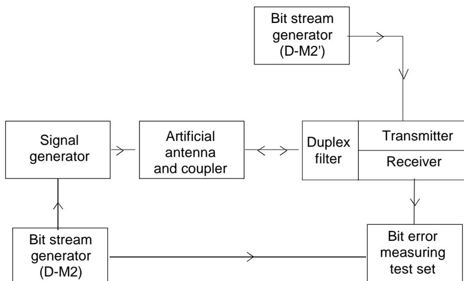
**Figure 33: Measurement arrangement**
