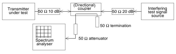
Figure 11: Measurement arrangement
