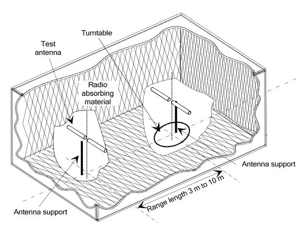
Figure B.1: A typical anechoic chamber
