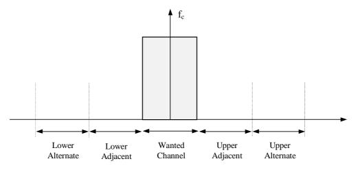
Figure 1: Adjacent and alternate channel definitions
