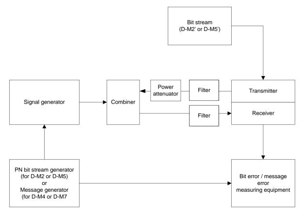
Figure 34: Measurement arrangement
