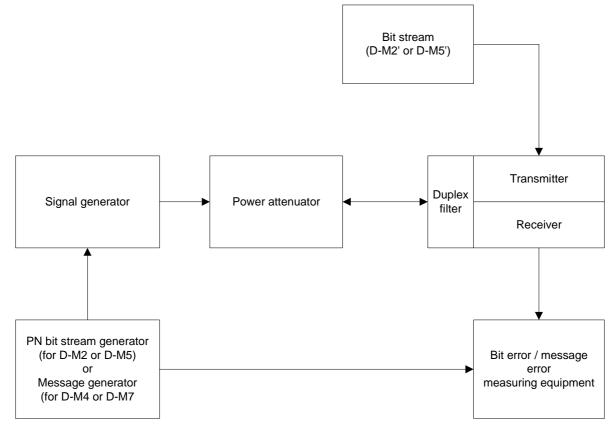
Figure 33: Measurement arrangement
