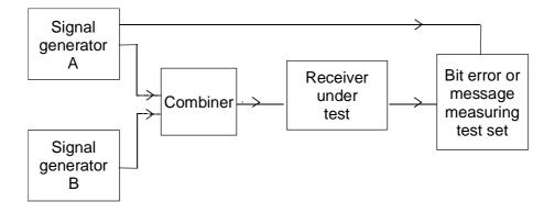
Figure 25: Measurement arrangement
