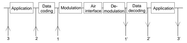
Figure 2: Test points for bit stream measurements
