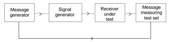
Figure 18: Measurement arrangement
