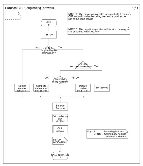
Figure 1: SDL for originating network dynamic description
