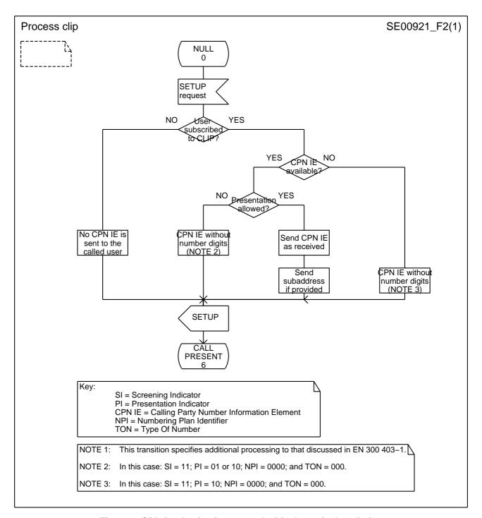
Figure 2: SDL for destination network side dynamic description
