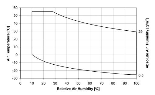
Figure 3: Climatogram for class 3.3: Not temperature controlled locations
