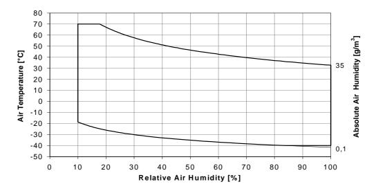
Figure 4: Climatogram for class 3.4: Sites with heat-trap
