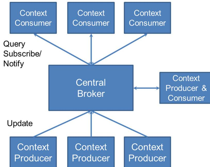
Figure 4.3.2-1: Centralized architecture
