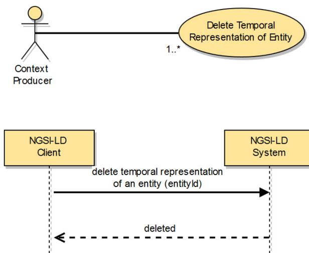
**Figure 5.6.16.2-1: Delete Temporal Representation of Entity use case**
