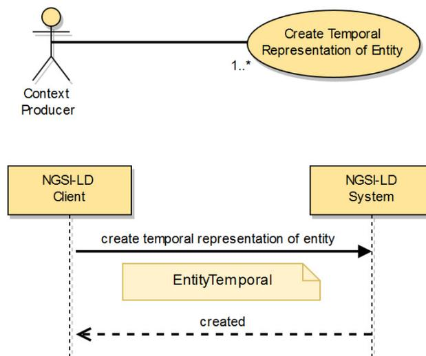
**Figure 5.6.11.2-1: Create Temporal Representation of Entity use case**
