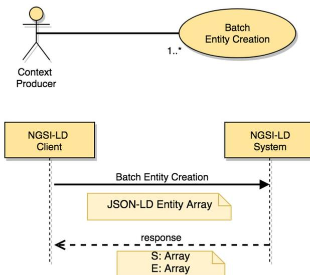
Figure 5.6.7.2-1: Create a batch of Entities use case
