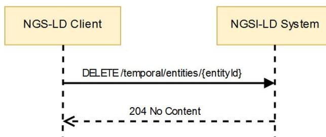
Figure 6.19.3.2-1: Delete Temporal Representation of Entity interaction
