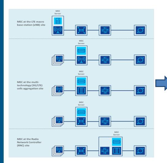
The multi-technology (LTE/3G) cell aggregation site can be located **indoor** or **outdoor**, for example:
