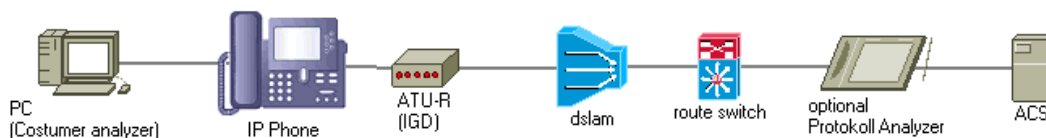
Figure 4.2-3 Test Setup for NONDSL Devices, connected over a DSL-Router
