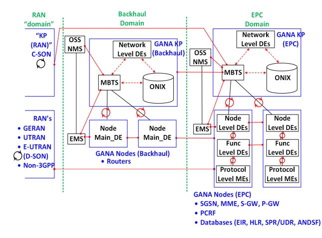
Figure 5: Interactions involving C-SON, and GANA entities for 3GPP Core Network and backhaul, to enable E2E Self-Optimization across network segments (figure extracted from [28])
