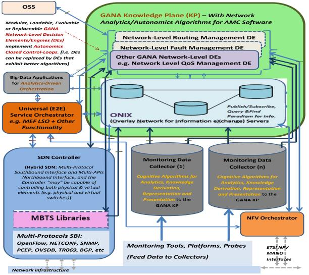
Figure 6: Core part of the unified framework for AMC, SDN NFV, e2e Orchestration, Big-Data driven analytics [13]
