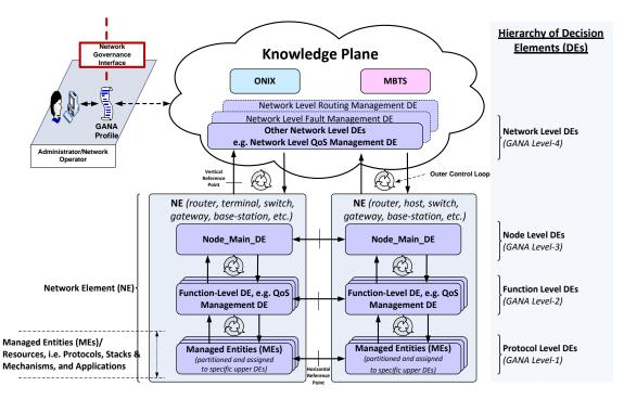
Figure 2: Snapshot of the AFI GANA Reference Model
