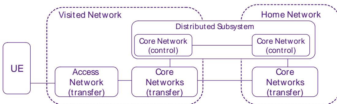
**Figure 3: NGN Network Distributed Subsystems (ES 282 001) [12]**
