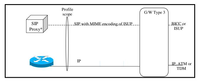
Figure 5: Profile Scope for SIP with MIME encoding of ISUP Interworking with BICC/ISUP with Type 3 Gateways
