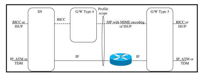
Figure 4: Profile Scope for SIP, with MIME Encoding of ISUP, Interworking with BICC/ISUP with Type 3 & 4 Gateways
