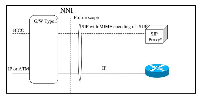
Figure 7: Profile for SIP, with MIME Encoding of ISUP, Interworking with BICC/ISUP with Type 3 Gateway
