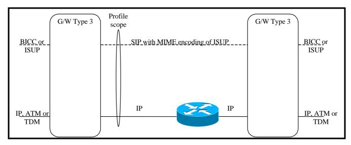
Figure 3: Profile Scope for SIP with MIME encoding of ISUP Interworking with BICC/ISUP with Type 3 Gateways
