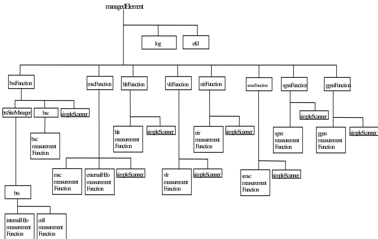
**Figure C.1: GSM 12.04 Performance Measurement Object Class Containment**
