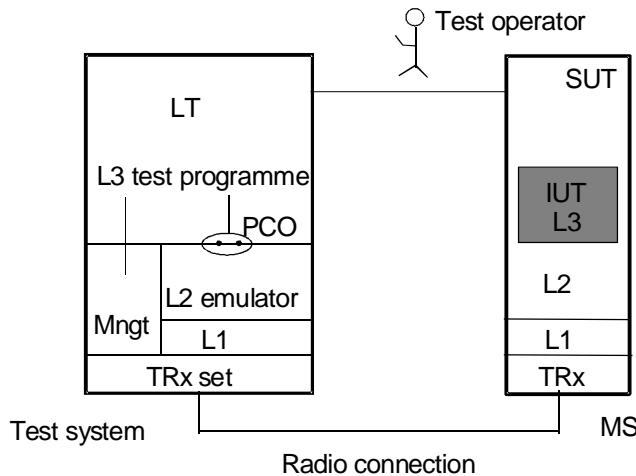
**Figure 3: Test system and distributed test method**
