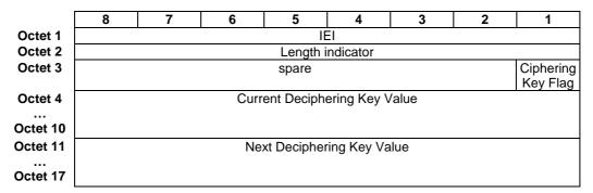
Figure 10.8.1/3GPP TS 49.031: Deciphering Keys IE
