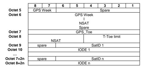
Figure 10.10.2/3GPP TS 49.031: Coding of Satellite Related Data
