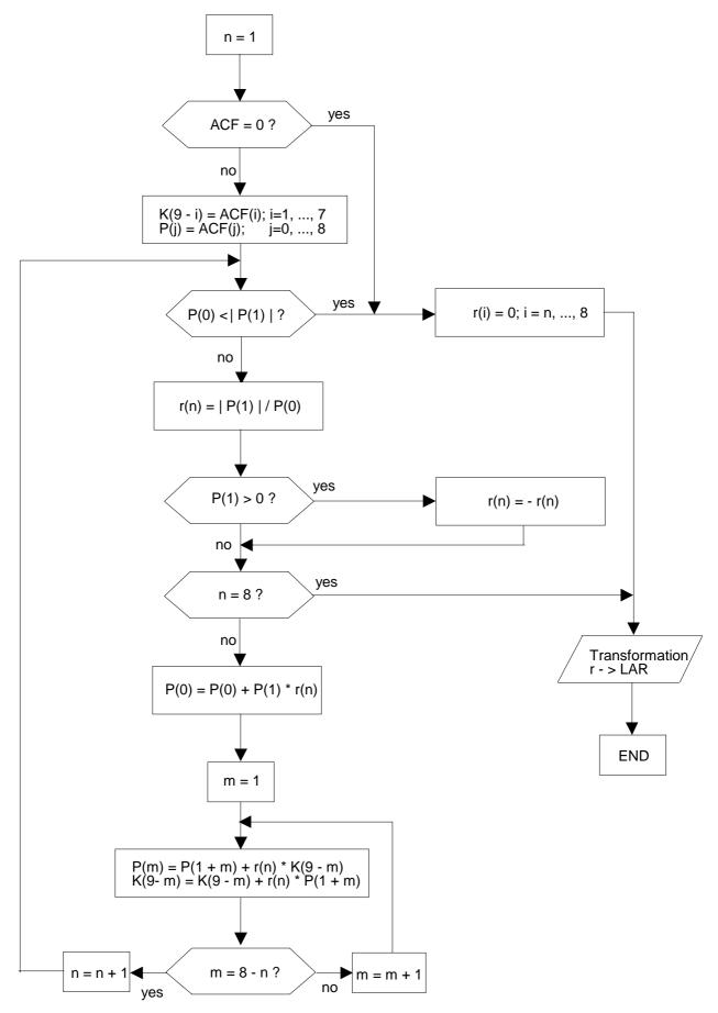
Figure 3.2: LPC analysis using Schur recursion
