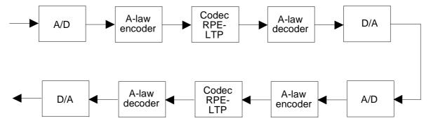
Figure A.1.2: Two - transcodings scheme (A-law)
