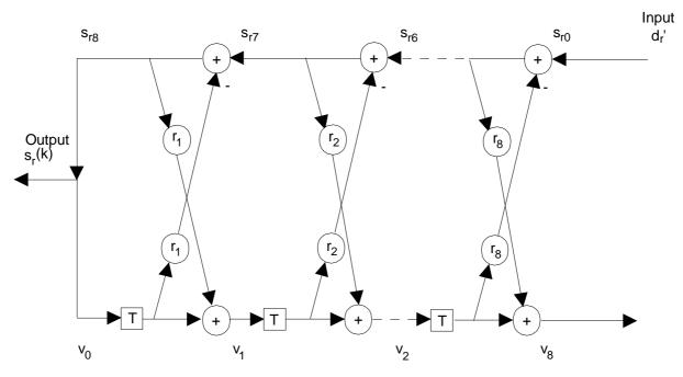
Figure 3.5: Short term synthesis filter
